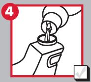
Pour the ready-to-use or diluted concentrate disinfectant into the electrostatic sprayer reservoir.
