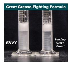
Add a drop of bacon grease and shake ten times. The suds level stays the same and the hazy water color is the emulsification – Envy's surfactants attacking the soil better.
