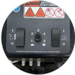
Self propelled with variable speed control
