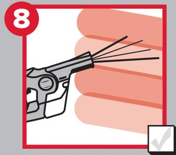
**8** When applying the solution, make sure you move at an even pace to ensure the surfaces are thoroughly covered. Apply solution using a **slow sweeping motion** across the surfaces and allow the spray to overlap when moving to the next section. Follow a continuous path through the room moving backward toward the door, spraying away from your body and not walking into the spray.
