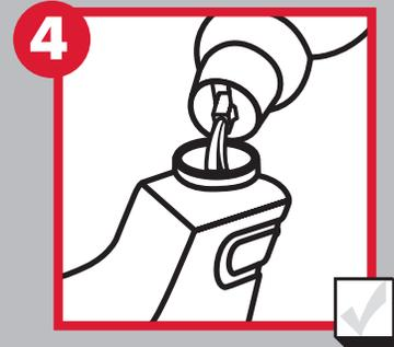
**4** Pour the ready-to-use or diluted concentrate disinfectant into the electrostatic sprayer reservoir.
