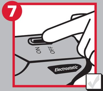
**7** Place the electrostatic spray function in the **ON** position. If the sprayer has the ability to change nozzles that impact particle size, set the size according to the spraying directions on the label. Position in a rear corner of the area to be sprayed. Using the sprayer, apply disinfectant evenly over the hard, non-porous inanimate surface to be cleaned, at the distance specified on the label. Make sure to cover surfaces evenly.
