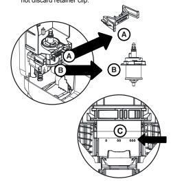
Push refill bag opening onto top of pump adapter post and push all the way down until fully seated and valve in refill bag opens.
