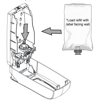
Ensure edges of refill bag are fully inserted into dispenser body and does not pinch bag when closing.
