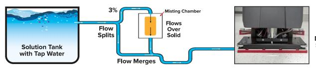
Cleaning Solution Delivered to **Scrub Deck**
