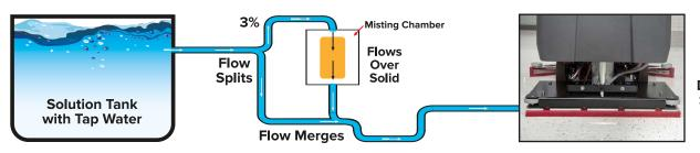
Cleaning Solution **Delivered to Scrub Deck**
