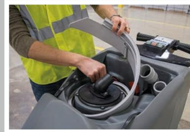
Brush Skirt and band clamp, located under recovery tank lid
